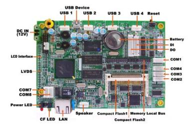
Features include 6xRS-232, 1x10/100 BaseT Ethernet capability, 16xDI, 16xDO, USB 1.1 4 host & 1 device, Optional configurable DIP switches, and 1-wire protection.
